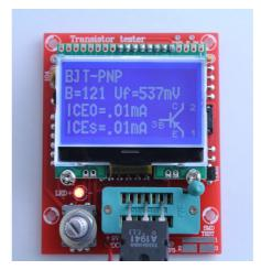
Display the Collector cutoff current Iceo with currentless base (10uA units) and Collector residual current Ices with base hold to emitter level. This values are only shown, if they are not zero (especially for Germanium transistors).
