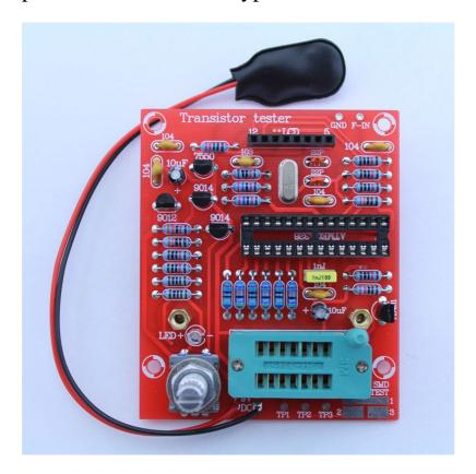
The welding direction of the LED: There is an aligned side that is the same with the PCB sign. Please note that the welding time of the LED should not be kept too long in case that the LED could be damaged.
