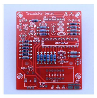
Next, weld the other electrical components based on , and please be aware of the type and direction of the transistor:
