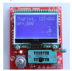
Thyristors and Triacs can only be detected, if the test current is above the holding current. Some Thyristors and Triacs need as higher gate trigger current, than this Tester can deliver. The available testing current is only about 6mA!
