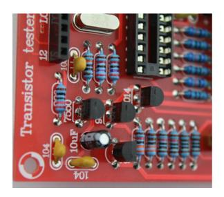
After all the welding jobs have been done, please connect the electric power instead of connecting Atmega328 and LCD(9V battery or external 5.5-12V DC power), and measuring the voltage of the pin7 and pin22 on the IC plug by using the multi-meter, and the voltage should be +5V(the button should be pushed when measuring), which means the circuit and power are working in normal condition.
