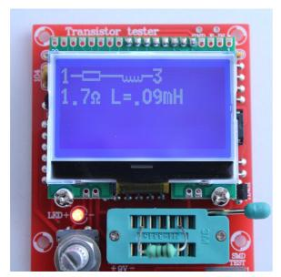
For resistors below  $2100\Omega$  also the measurement of inductance will be done. The range will be from about 0.01mH to more than
