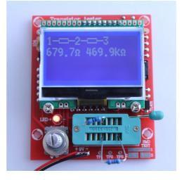
Up to two Resistors are measured and shown with symbols and values with up to four decimal digits in the right dimension. All symbols are surrounded by the probe numbers of the Tester
