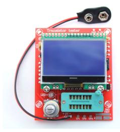
After all the installation, connect the power(9V 6F22 battery,or 5.5V-12V DC power). Push the button, you will see the character. Congratulations, the gadget could be put in use!
