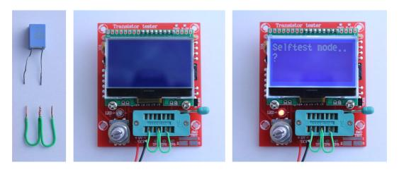
You should not touch to any of the test ports or connected cables when calibration is done. But the equipment should be the same, which is used for further measurements. Otherwise the zero offset for capacity measurement is not detected correctly. The resistance values of port outputs are determined at the beginning of every measurement with this option.
