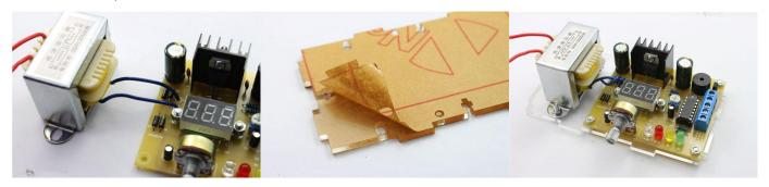
6. The red line of the transformer shall connect the power source of 200V; protect the welded power line with heat shrink tubing.
