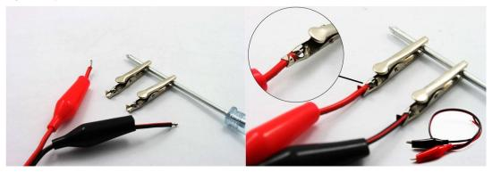
8. Anode and cathode of power source: output end of the adjustable power supply.
