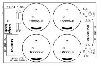
Led1 is + power indicator, led2 is – power indicator, R1 and R2 are current limited resistors.
