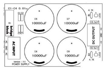
Led1 is + power indicator, led2 is - power indicator, R1 and R2 are current limited resistors.
