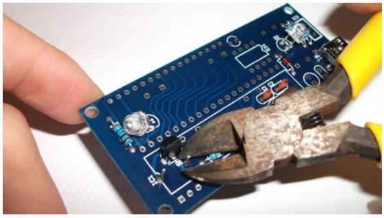
Adjust the transistor as shown:
