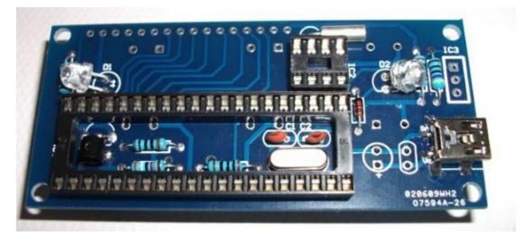
7. 100UF electrolytic capacitor and 104 ceramic capacitor soldered:
