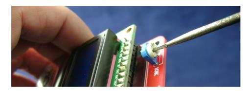
After all the installation, connect the power supply, right adjust the resistance 10K and you will see the character.
