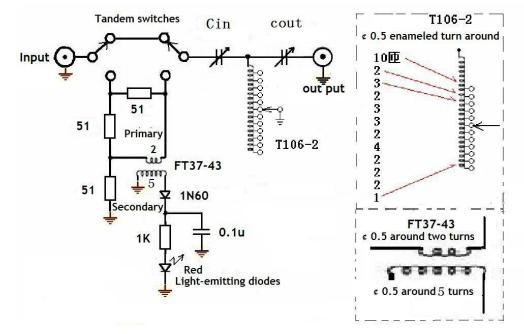
1, the following circuit diagram the two magnetic labels are wound in the figure.
